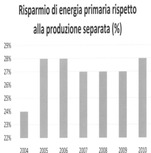
Figure 25: Energy savings from CHP as compared to separate production of electricity and heat (Mtoe)
