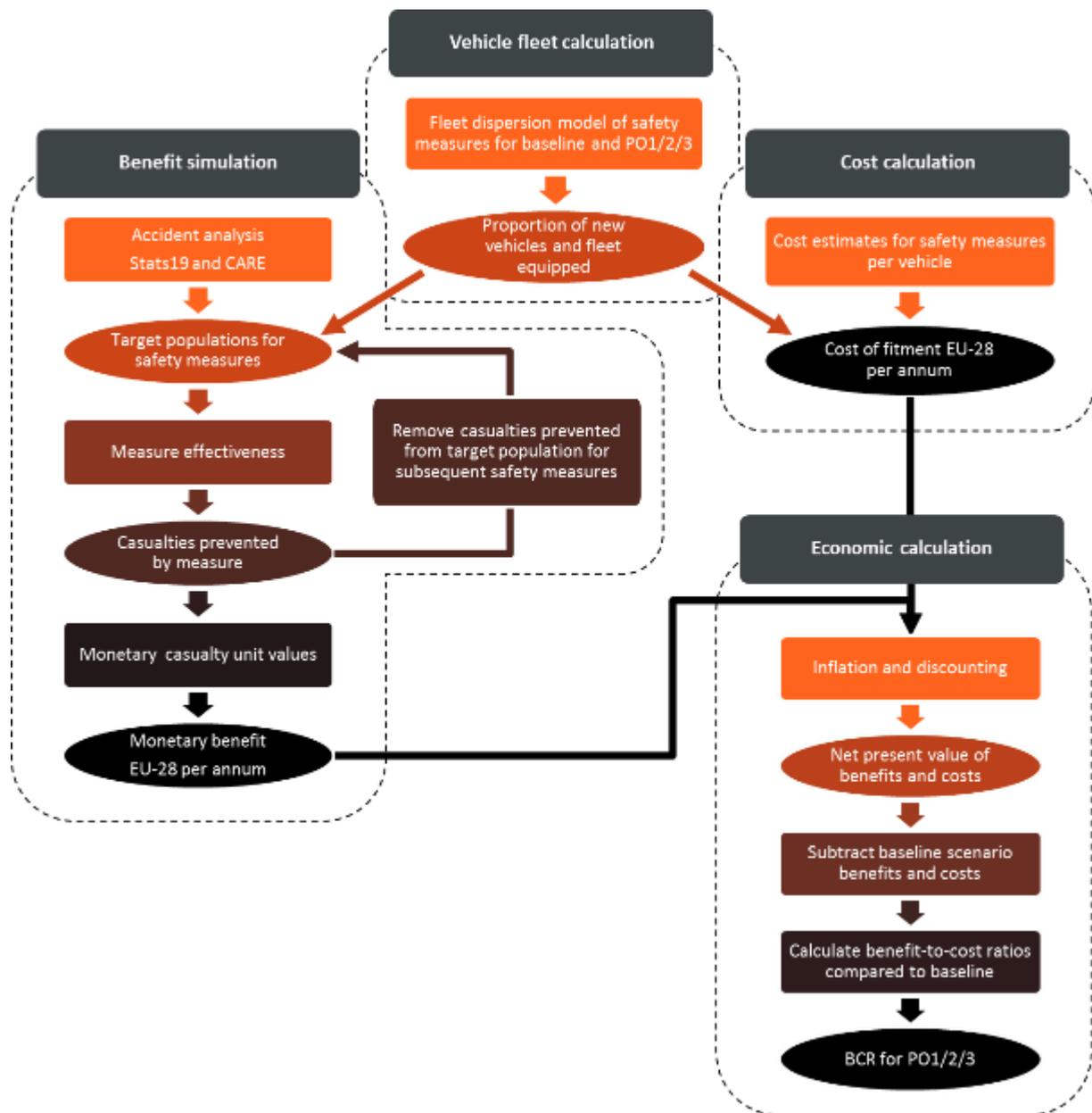
**Figure 25: Flowchart of the simulation model to calculate benefit-to-cost ratios (BCRs) for policy options PO1, PO2 and PO3, respectively, compared to the baseline scenario**
